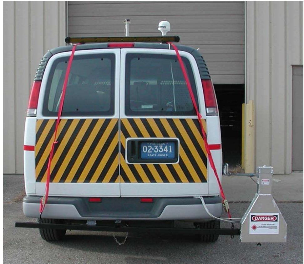
Figure 2.4.9 High Speed Underclearance Measurement System
